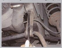
Next we unscrewed two M8 bolts securing antiroll bar to each of the two chassis longitudinals. They may be seized in their threads, so take care not to break them, spraying with penetrating oil and then winding them a little way back in again
