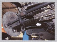
And that's about it. Check all the nuts and bolts for tightness and refit the wheels, have the front-end geometry reset, and you'll be ready to go. New balljoint may last no longer than original, but replacing it if and when necessary should now be a 20-minute job - or even less! Now to tackle those oil leaks...
