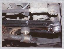
In earlier cars anti-roll bar is attached to steel suspension arm by means of aluminium casting with rubber insert, but later 944 and derivatives - and the 968 - has a simpler eye-and-stud arrangement. This leaves you with two routes
