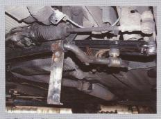
To fit anti-roll bar (here with set of new bushes) first offer up eye and stud at each outer end through newly drilled holes in suspension arms, with rubber bushes above and below. Or fit those aluminium bracket-and-bush assemblies. Next attach 'L'shaped brackets to the chassis and tighten bolts
