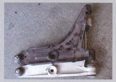
And this shot shows how Porscheshop has modified Golf-style steel arm to fit any of the later cars including 968: £135 each. Note laser-cut (and TIGwelded) plate to place ball-joint in correct position, plus modified rear mounting point to the chassis
