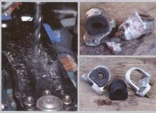
Drill new steel arm for single eye-bolt, or else buy a set of new 9245-style brackets and bushes (above, right). They're pricey, though (about £30 a side all in; steel control arm costs only around £15) and can subsequently corrode quite badly, as shown here
