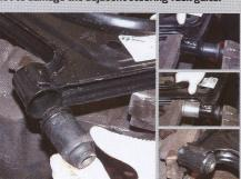
New bush for front mounting is pressed into eye on arm. Make sure it goes in the right way round, and help it on its way with WD-40. Socket provides clearance for end of the bush as it starts to emerge from the eye - but don't push it through too far
