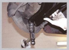
Begin fitting new suspension arm by tapping balljoint pin upward into eye at base of stub axle. Don't use excessive force, though. If it's tight find out why - surface rust, perhaps - and maybe repeat that wedge trick with a screwdriver blade or similar
