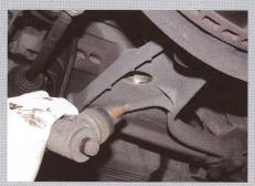
First step in replacing our car's arms was to remove anti-roll bar by undoing M8 nut securing each connecting link up through moulded recess. Broken stud on one side meant we ended up replacing that entire assembly - and rubber mounting bushes, too
