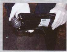
The original-equipment steel arm has ball-joint secured to its outer end by three rivets, but after-market replacements such as this use conventional bolts, washers and locknuts. Make sure they're tight, but not over-tight
