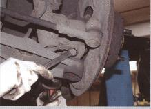
Grooved pin on ball-joint is secured into stub-axle assembly by means of an M10 pinchbolt (17mm spanner) and locknut. Here Porscheshop's Gavin Burns is using an impact wrench to loosen locknut, but ordinary socket wrench (and breaker bar) will do
