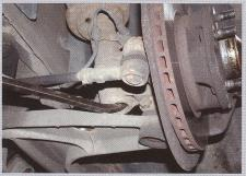
To confirm wear in bottom ball-joint place a bar between base of strut and control arm - whether steel or aluminium - and lever them apart. Even slight movement will be obvious. Don't be misled by loose wheel bearings or worn dampers, though
