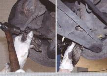
With locknut removed the pinchbolt can be driven forward through stub-axle forging by means of first a hammer and then a hammer and punch. Yellow paint suggests that this is the first time this one has been disturbed in this car's 170,000km to date
