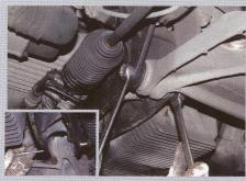
Front end of each arm is attached to engine-bearer crossmember by a single M12 (19mm spanner) bolt and self-locking nut. Former is then driven forward, again with a punch if necessary - but do be careful not to damage the adjacent steering-rack gaiter
