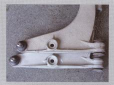
Close-ups make it clearer still. Here you can see difference in length between early-type (top) and late-type (bottom) aluminium arms. The apparent increase in wheel track was prompted by switch to negative-offset steering (see p107)
