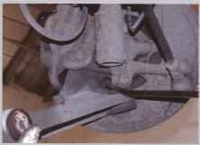
To detach control arm first pull it straight down away from chassis mounts, and then use a prybar to lever pin out of stub axle. This shouldn't be tight, but if it is all you need do is gently drive a suitable wedge - a screwdriver, perhaps - into vertical slot
