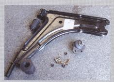
This is all the hardware we needed to convert each side of our 1985/2 944's front suspension to the earlier type, with a pressed-steel control arm and a replaceable ball-joint. Arm is exactly the same as a Mark 1 Golf's, and fits either side of both vehicles
