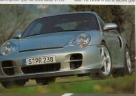
Front apron is more space than plastic, with massive central intake, and just one borizontal slat in each 'nostril'. Note additional vent between bumper and bonnet
