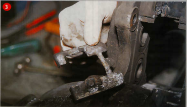
Once the screws are out of the way the plate should be free to move. But you might still need to lever it away from the caliper using a screwdriver (take care not to damage the aluminium, though). Our 964's calipers weren't badly corroded but, as you can see, the plate has clearly seen better days and is fit only for the bin
